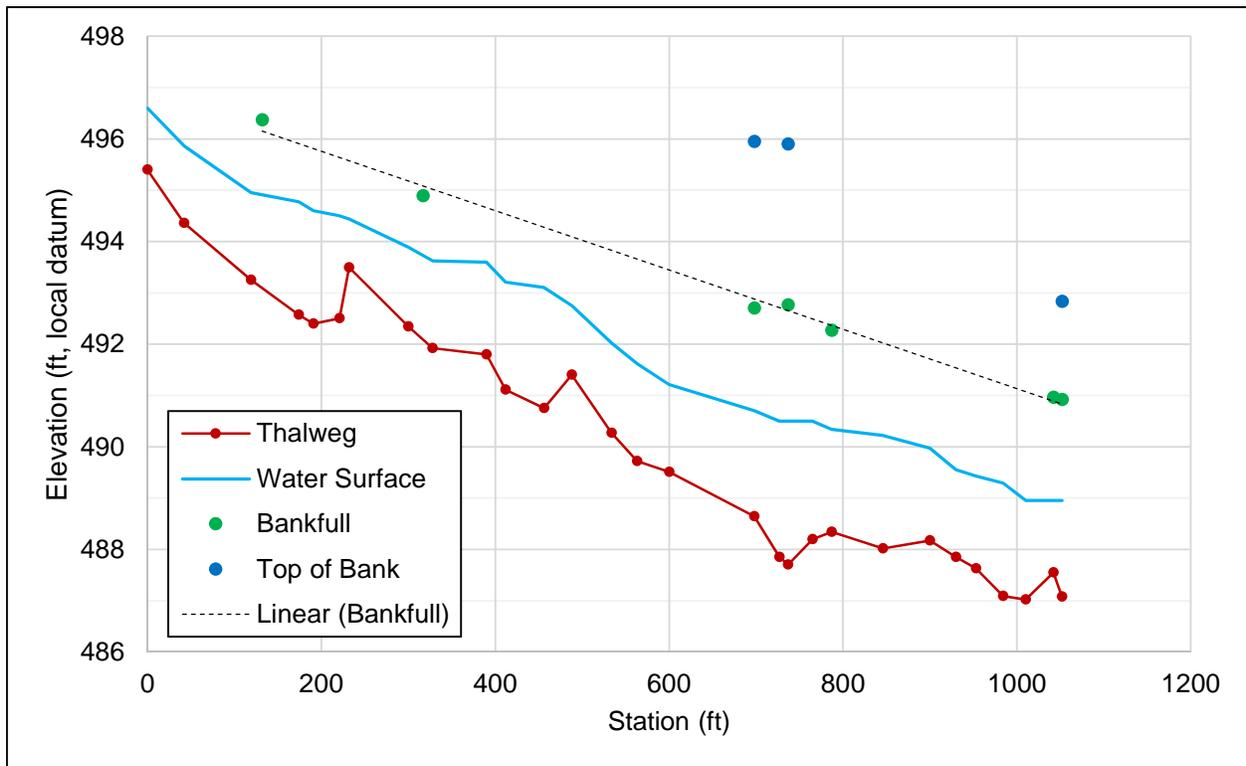
Figure 26. Longitudinal profile through Fox Creek Reference Reach.
