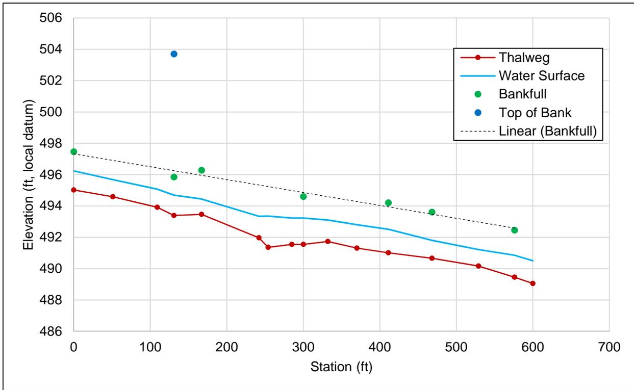
Figure 17. Longitudinal profile through Wood River Campground Reach.
