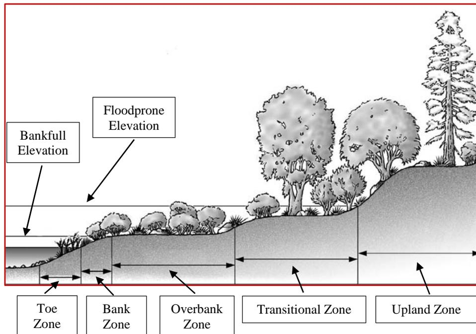
Figure 122. Profile view of typical bank zones.
