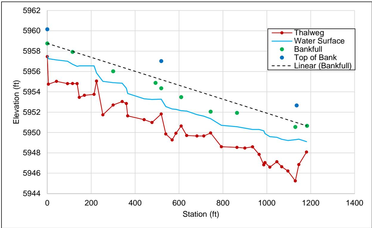
Figure 32. Longitudinal profile through Training Channel Reach.
